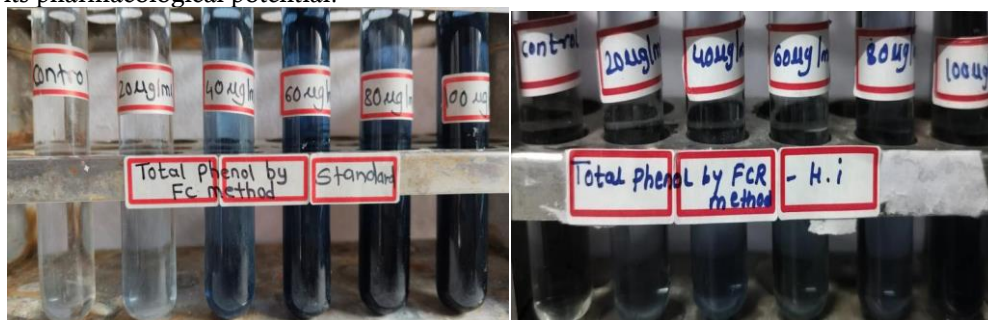
Figure 3.2: Total phenolic content estimation using Folin–Ciocalteu method showing standard (gallic acid) and Helicteres isora fruit extract at different concentrations
