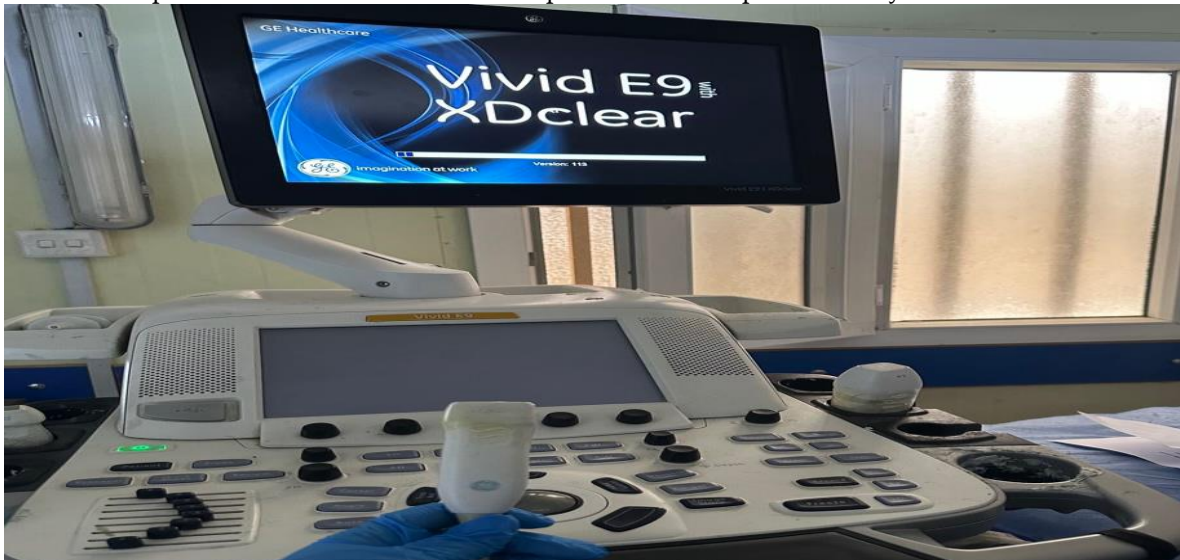
Figure 2.1: A GE Medical Systems Vivid 9 ultrasound machine equipped with a 1.5–5 MHz sector transducer probe
