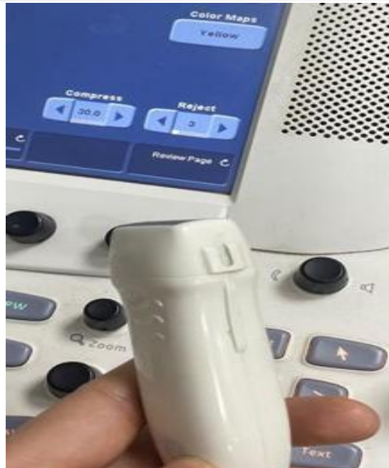
Figure (2-10) VIVID9 GE Probe with a 3.5 MHz transducer. Made in Norway by GE Vingmed Ultrasound, 2012.
